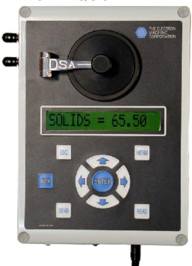
The DSA E-Scan is an automatic, benchtop critical angle refractometer with a digital readout and heated sample chamber. It measures the critical angle of refraction of sample fluids which are directly correlated to various measurements including percent dissolved solids. The instrument is equipped with a menu-driven user interface and is factory calibrated and temperature compensated. The measurement is not affected by opaque liquids or suspended solids making it ideal for black liquor.
