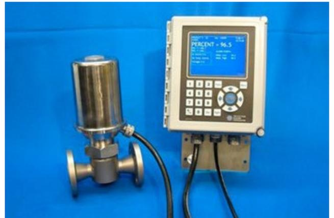
Based upon the refractive index (R.I.) of a given aqueous solution, the MPR E-Scan can determine the concentration of the solution and relay that value in real time for proactive process control.
